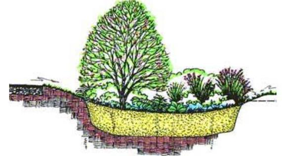
Bioretention areas are depressions constructed to treat stormwater as it flows through vegetation and soil before entering the storm drainage system. Parking lot islands are good candidate sites for bioretention.
