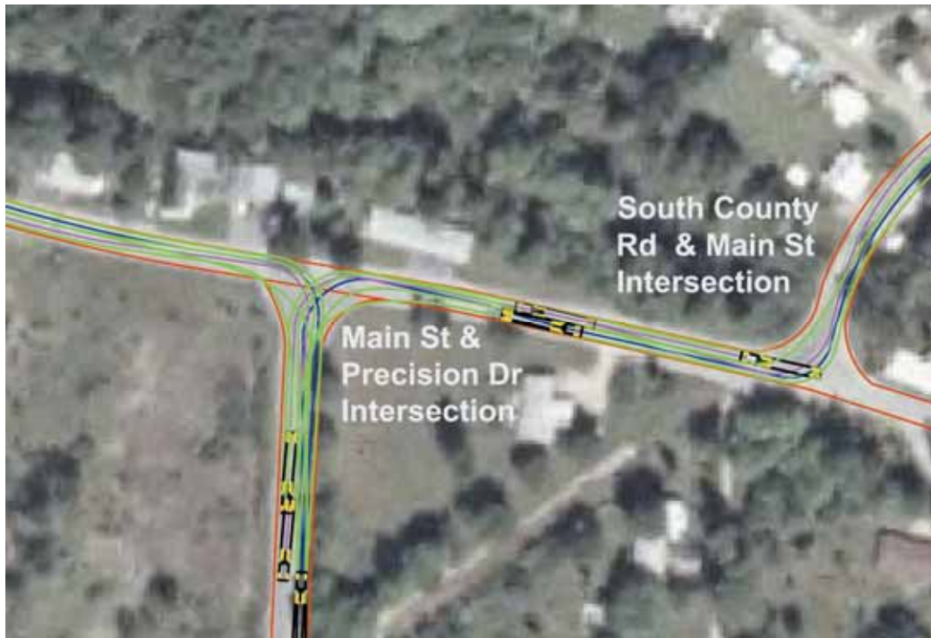
Figure 4: Turning Movement of WB-67 at Main Street Intersections with Precision Drive and South County Road
