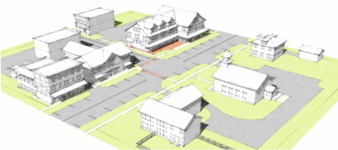
THIS: SHARED PARKING LOCATED TO THE REAR OR SIDE OF BUILDINGS WITH CROSS ACCESS BETWEEN LOTS
